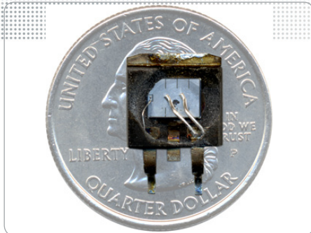
Figure 3 Test MOSFET with burned spot. Plastic casing has been etched away to reveal MOSFET die, and lead wires.
