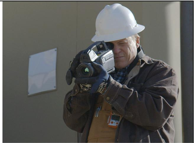
*Ensure safer working conditions and a more efficient facility using an OGI camera to look for dangerous leaks at safe distances.*
