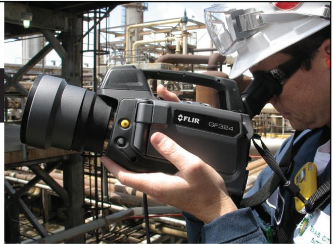
Check for hydrogen leaks from many components in a power generation facility with the GF343 while using CO<sub>2</sub> as a tracer gas.
