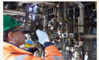
Dave Fashimpaur from BP is checking for leaks of natural gas using his GasFindIR HSX
