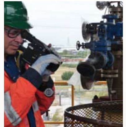
Dave Fashimpaur from BP is checking for leaks of natural gas using his GasFindIR HSX
