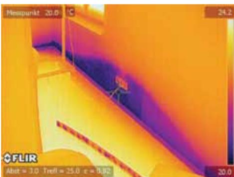
This case of water damage clearly shows the advantage of the Picture-in-picture feature, since the client can quite easily see where this thermal image is located, while this would be more difficult with only the thermal image.
