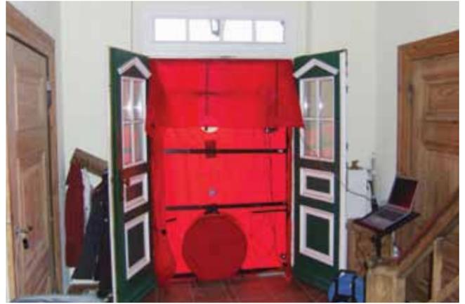
A Blower Door test consists of a ventilator that's installed in a doorway, sucking air out, which causes the outside air to rush into the building through available cracks and crevices.
