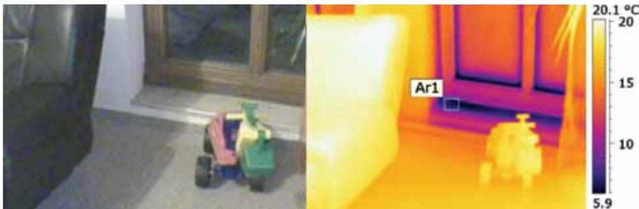
*This Blower Door test clearly shows that there's air leakage at the windowframe.*
