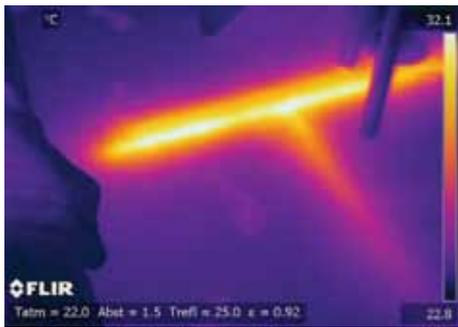
This thermal image shows where the warm water pipe has been installed beneath the floor.
