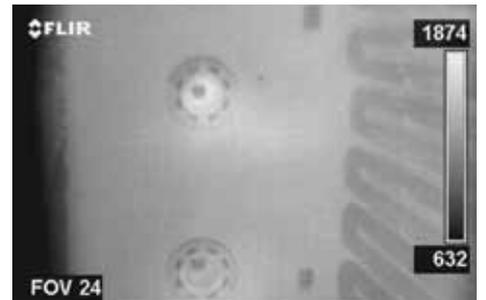
Due to the built in flame filter the FLIR GF309 thermal imaging camera can see through flames and even measures the temperatures behind the flames.
