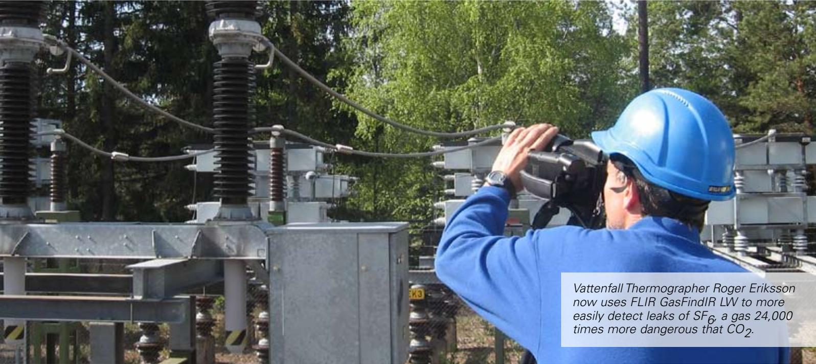
*Vattenfall Thermographer Roger Eriksson now uses FLIR GasFindIR LW to more easily detect leaks of SF<sub>6</sub>, a gas 24,000 times more dangerous than CO<sub>2</sub>.*
