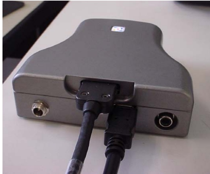
Figure 16: IEEE-1394 Cable connect to Firewire Module
