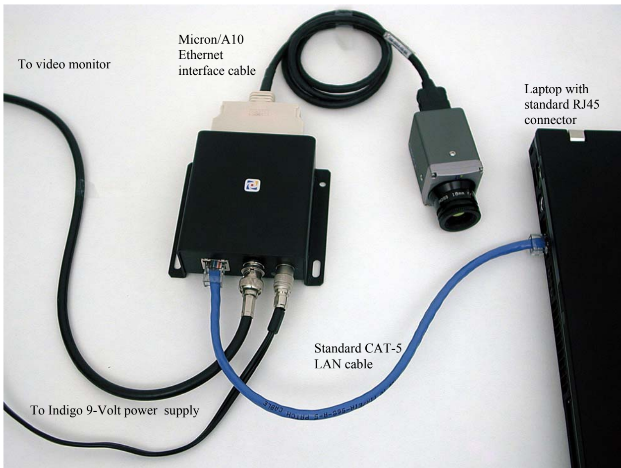
Figure 7: Laptop connected to Micron/A10 and Ethernet Module
