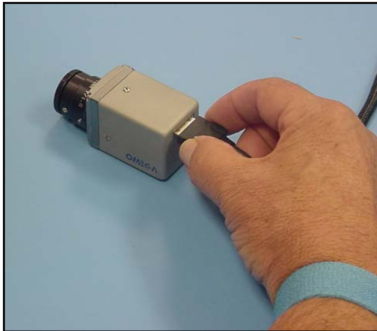
Figure 4: Connecting the Interface Cable to the Micron/A10
