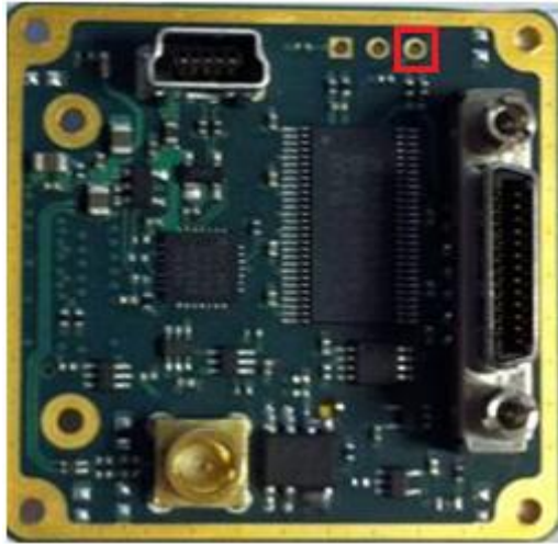
Figure 19: Ext Sync Header Connection
