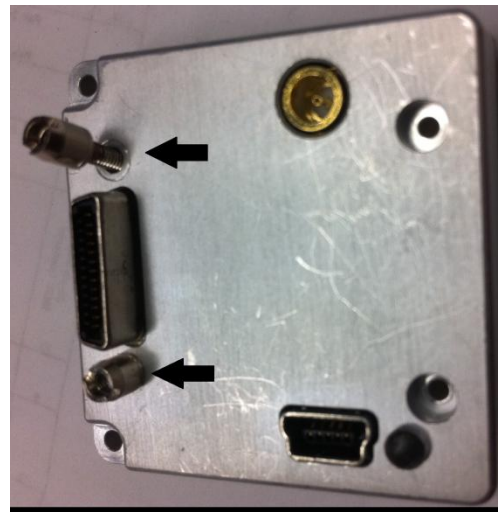
Figure 12: Jack Screws to remove
