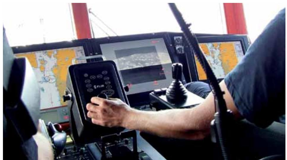
In the Stormbull's cabin two multifunction displays and one dedicated display give all three crewmembers continual access to the Voyager's thermal images. The ergonomic Joystick Control Unit (JCU) is mounted in the middle.
