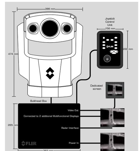
Schematics of the installation of the Voyager aboard the RS 146 Stormbull.
