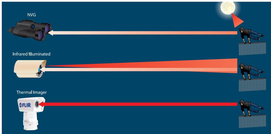
This illustration demonstrates the relative strengths of each imaging technology. NVGs (top) and Infrared Illuminated cameras (center) both require outside illumination which weakens as it nears the camera. Thermal security cameras (bottom) generate images regardless of available visible lighting, and do not lose strength nearly as rapidly as the other two technologies.
