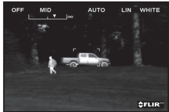
When a heat source can be classified as human, it stands out from other objects in the scene.
