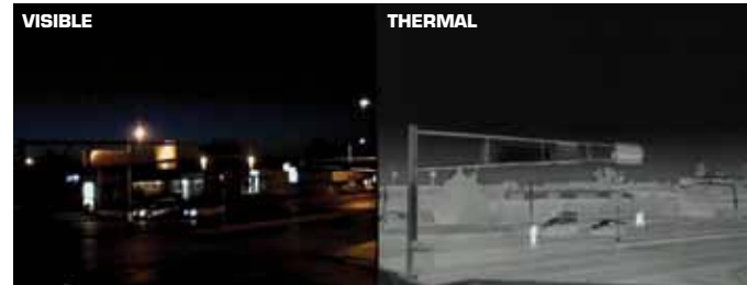
Thermal cameras can see cars at the stop bar and pedestrians in the intersection clearly in the dark.
