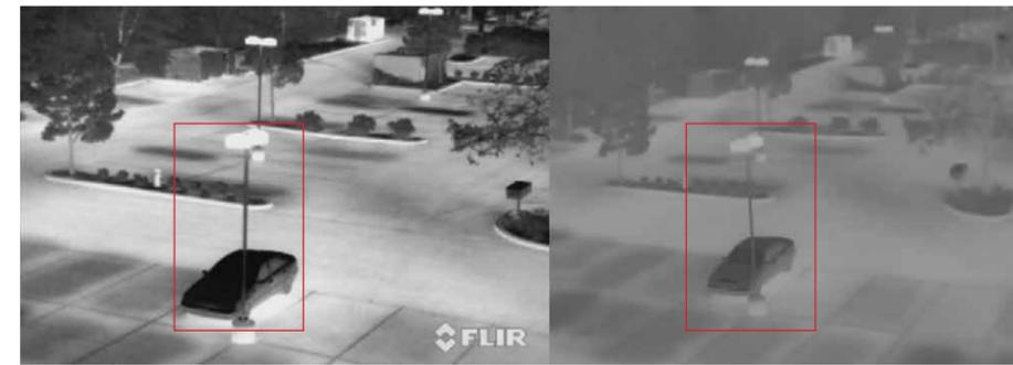
The other side of the coin is even more dramatic. These images were taken at midnight, when things have become more uniformly cool. Again, the FLIR maintains its image contrast and detail, while the Axis image has suffered noticeably on both counts and produces a flat, washed-out image.
