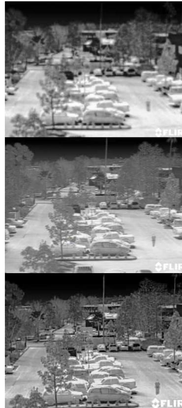
These three images were captured with a 160x120 thermal camera (top), a 320x240 camera (middle), and 640x480 camera (bottom). The 640 resolution camera shows more detail and allows the viewer to see things from farther away, than its lower resolution counterparts.
