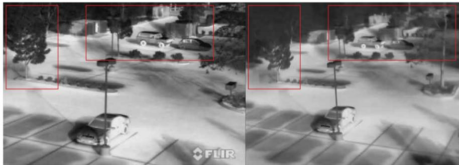
This set of images was taken at 6PM. The FLIR image (on the left) has greater contrast, shows more small details (take particular note of the areas outlined in red), and is in focus throughout the entire depth of the image. These points are notable because this is one of the times of the day that can be most challenging for thermal imagers. Remember that thermal cameras don't just make pictures from heat; they make pictures from tiny differences in heat.
