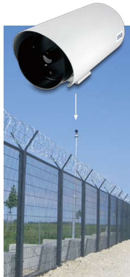
Twenty-two FLIR Systems SR-35 thermal imaging cameras were installed along the eleven km long fence
