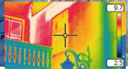
A former window - closed with bricks or plaster of a better quality
