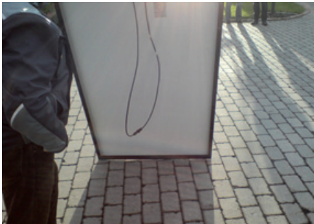
These images taken from the back of the same solar panel show much less reflection than the front, making the temperature measurements much more accurate.
