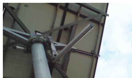
Inspection from the back shows no hot spots, the hot spots in the previous thermal image taken from the front were caused by reflection.
