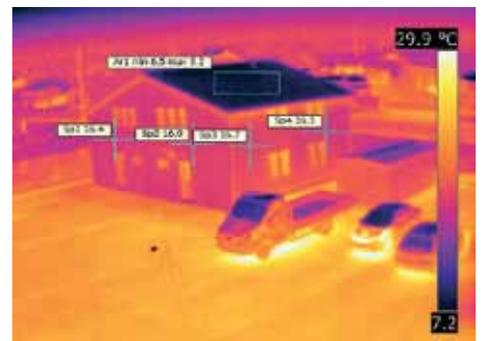
*The roof remains cold, even though one of the apartments is heated ( $\Delta T = 13^{\circ}\text{C}$ ). The ridge-tile appears at the same temperature than the roof, which is a sign of well insulated roof.*
