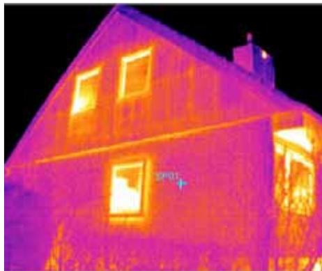
*This thermal image shows an example of insulation failure in a residential building that is used in Rockwool's thermography course.*
