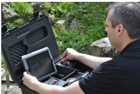
With the FLIR thermal imaging camera mounted on a pole, the wireless connection is perfect for this application. The thermal images can be viewed on the tablet PC and the camera can be controlled remotely using the FLIR app
