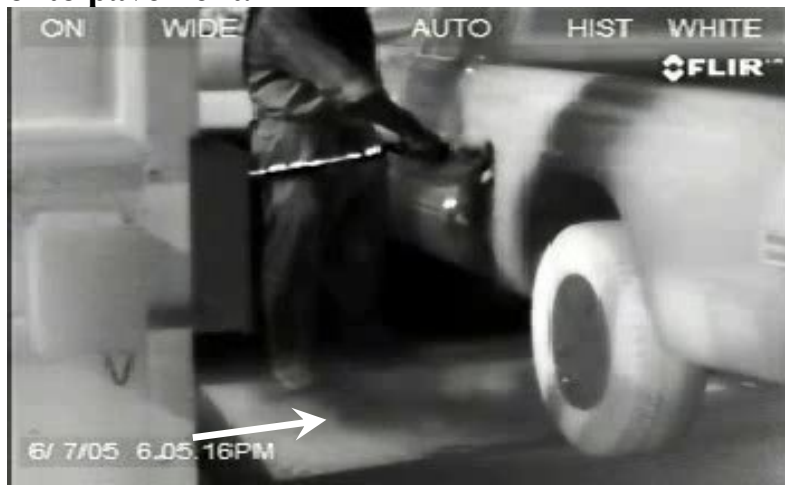
Figure 11, Gasoline fumes cascading from fill spout onto pavement.
