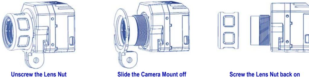
When installing the Camera Mount, be sure to engage the two alignment pins with the corresponding holes on the camera body.
