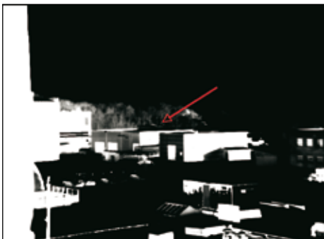
Picture 6: narrow span in the middle of the dynamic range pointing out pixel sized targets in the woodlands – humans?
