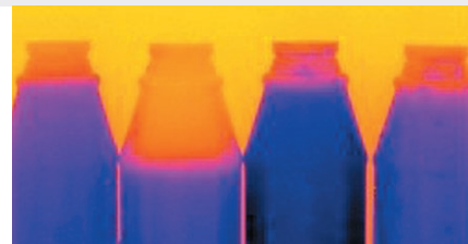
Detecting liquid levels in visually opaque bottles.
