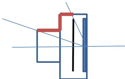
**Figure 1: Radiation from the parts in red is not subtracted after an internal FFC.**
