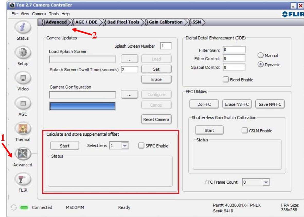
Figure 3: FLIR Camera Controller GUI – Advanced Tab
