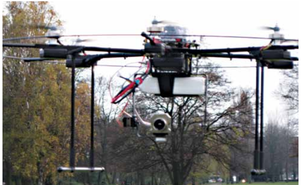
Due to the Tau thermal imaging camera core this UAV can be very effectively used to search for missing persons, even at night.
