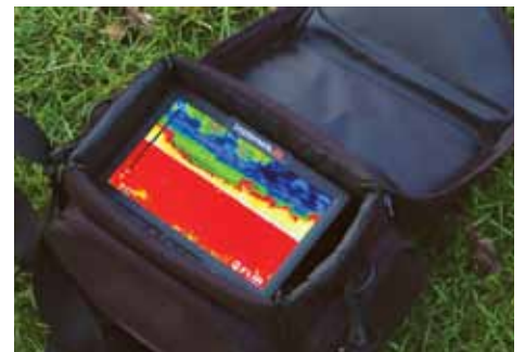
The thermal images are sent through a wireless video down-link to the transfective TFT monitor supplied by Coptersale.de.
