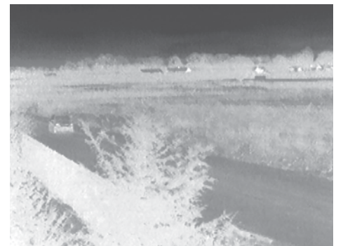
A car seen from the hexacopter at a distance of approximately 256 meters, using a 640 x 480 FLIR Tau thermal imaging camera.
