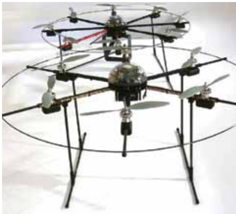
Coptersale.de delivers both hexacopters (with six rotors) and octocopters (with eight rotors).
