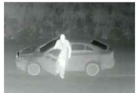
A man stepping out of a car as seen by a 640 x 480 FLIR Tau thermal imaging camera. The hexacopter is hovering at a height of 9 meters and at a distance of approximately 54 meters.
