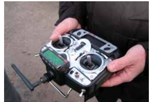
With the remote control unit the pilot can control all of the hexacopter's movements.
