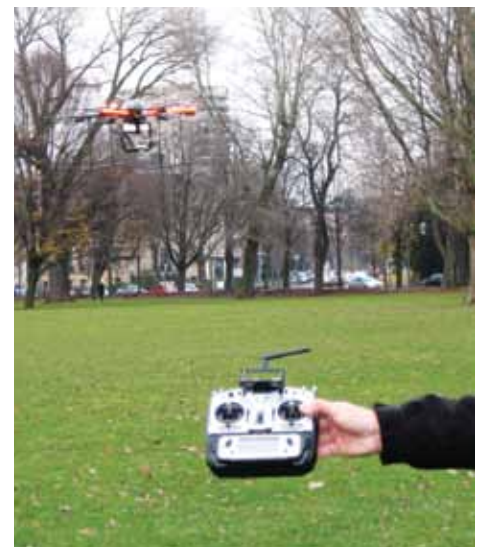
If the copter receives no information from the controller it will use the information from the elevation meter and GPS system to hover in the same location.
