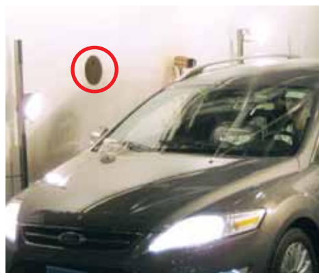
The thermal imaging camera behind the hole records the temperature of the air coming out of the air conditioning vent.
