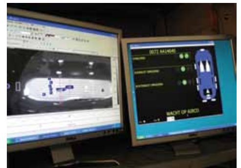
The programmable logic controller (PLC) compares the measurement data from the thermal imaging cameras with previously defined parameters.
