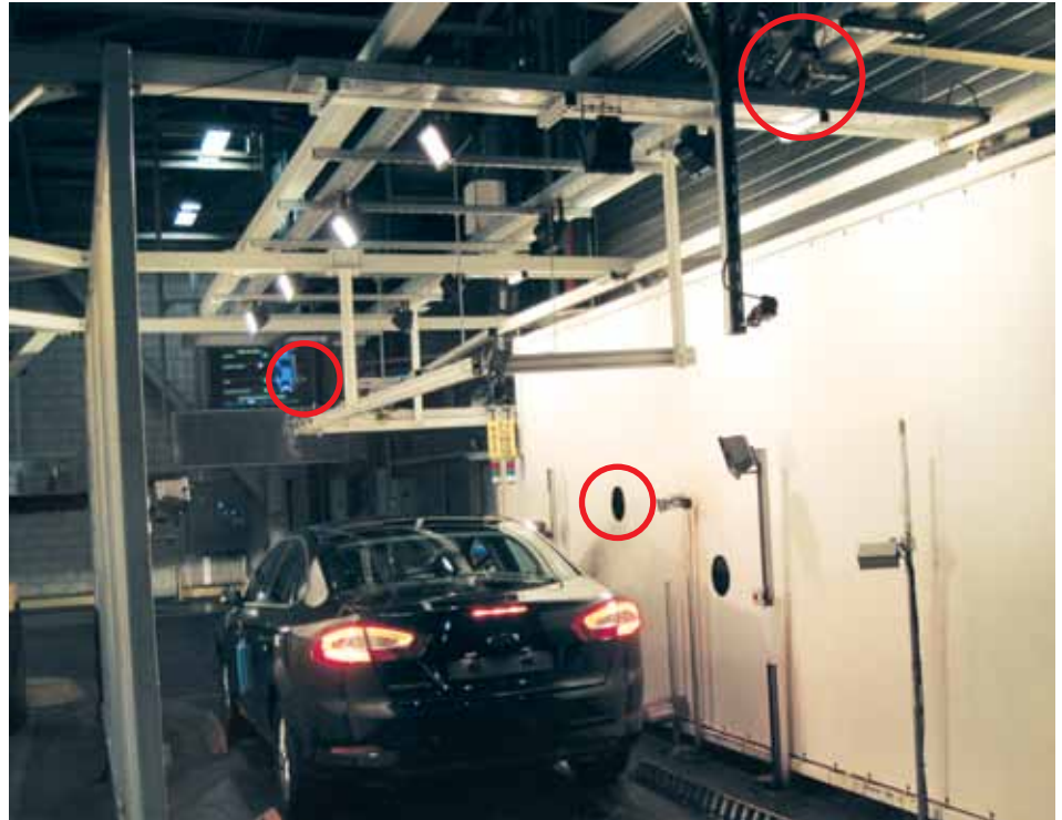
Ford Genk has three FLIR A320 thermal imaging cameras for testing the front window heating system, the rear window heating system and the air conditioning system. The locations of the thermal imaging cameras are marked in red.
