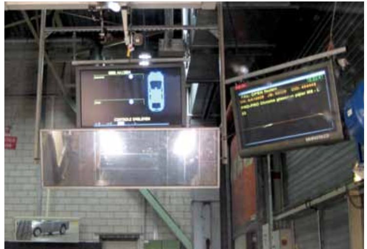
The screen next to the FLIR A320 thermal imaging camera that's pointed at the front shows the progress of the test.
