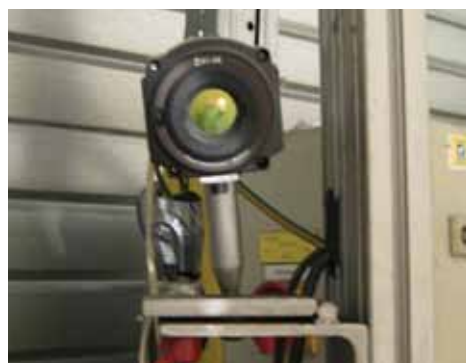
This FLIR A320 thermal imaging camera is used to check the air conditioning system.
