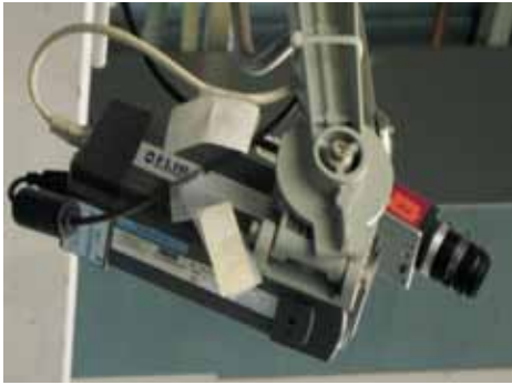
This FLIR A320 thermal imaging camera is used to check the rear window heating system for defective heating elements.
