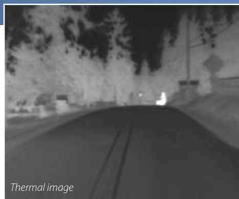
A FLIR Systems thermal imaging camera produces a crisp image in total darkness. The bump in the road is clearly visible on the thermal image but can not be seen with the naked eye.
