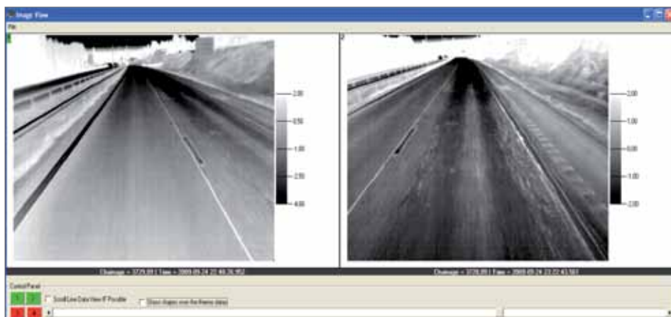
Good quality pavement (figure on left) provides a very homogenous thermal image while the thermal image to the right shows signs of cracks and water ingress in the asphalt.
