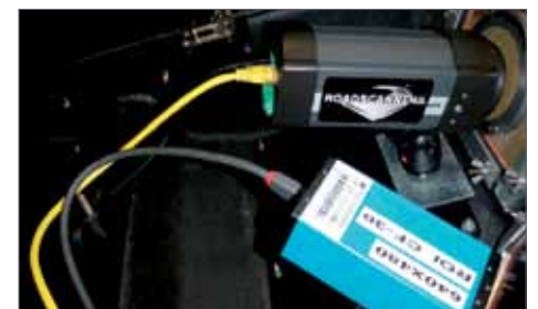
The Road Doctor diagnostics top box contains both a FLIR A-Series thermal imaging cameras and a digital video camera.
