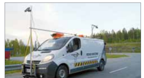
This special setup to check bridges includes an A-Series camera with a 90° wide angle lens attached to the front pole and a laser scanner on the rear pole.
