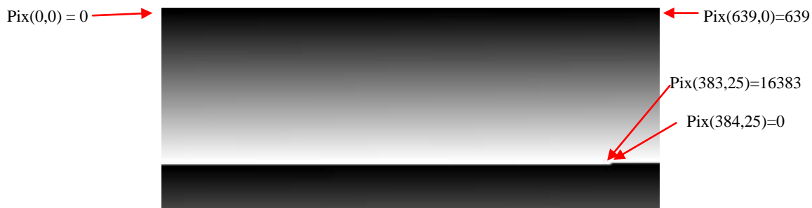
Figure 17: Ramp test pattern example for Top Portion of Ramp Image (Digital values shown apply to the optional 14-bit digital data stream.)
