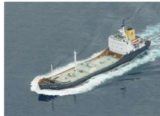
The M.V. Golden Bay: a cement carrier with a capacity of 4,500 tonnes.
