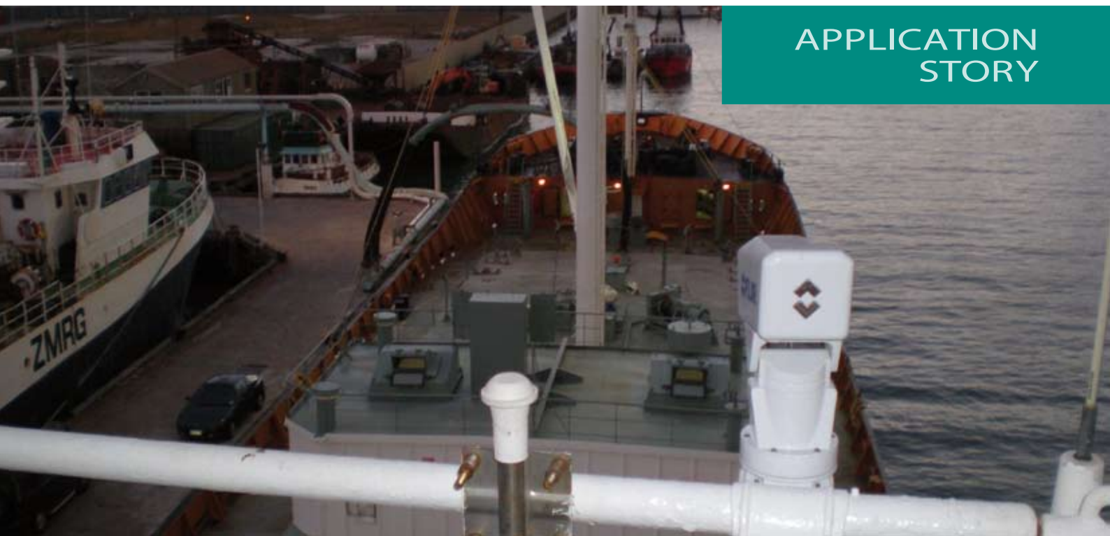
The FLIR Systems Navigator Pan / Tilt was installed just above the bridge of the M.V. Golden Bay. It helps the crew to avoid deadly accidents.
