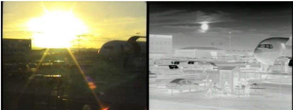
Figure 3: Backlit daylight camera on left; thermal camera on right
