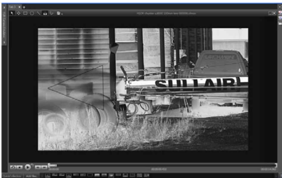
This image shows the vapor/exhaust exiting the rear of the cannon after the shot. The triangular dark area within the triangle is not a cold area on the building, but actually supersonic airflow—this pumpkin actually broke the sound barrier (343.2 meters per second, roughly 768 miles per hour) complete with sonic boom. Without IR imaging, it is impossible to even see the pumpkin leave the cannon with the naked eye, it's moving so rapidly.
