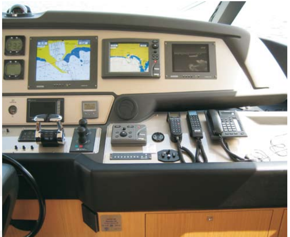
The joystick to control the FLIR Systems thermal imaging camera and the LCD display on which the thermal images are displayed are esthetically integrated in the bridge of the Ziacanaia
