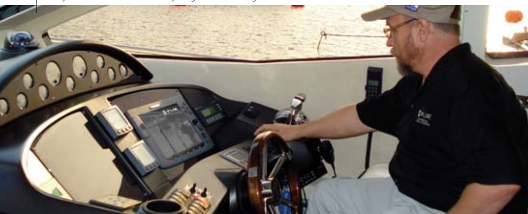
The thermal images produced by the FLIR Systems Navigator Pan/Tilt are displayed on a standard LCD. The Joystick Control Unit is esthetically integrated in the bridge.
